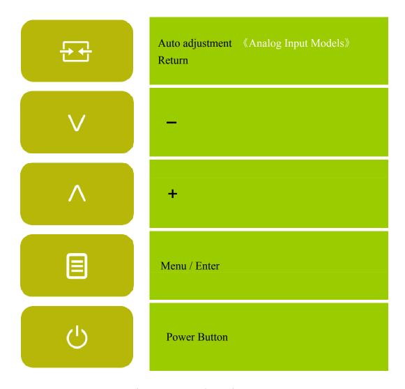
Figure.4. Control Panel Buttons
