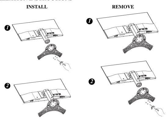
Figure.1. Installing and Removing the Base
