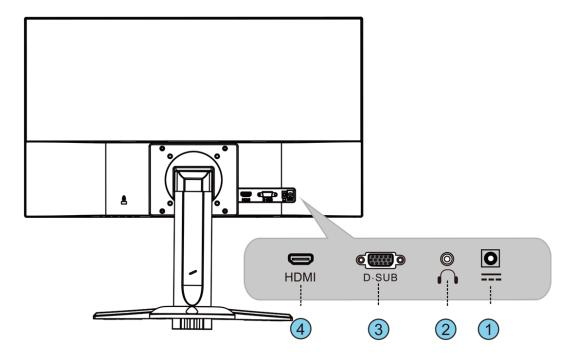
Figure.2. Connecting to a PC
